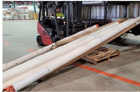
UNSUPPORTED & TOP HEAVY PALLETISED FREIGHT
