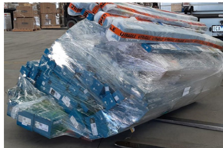
UNSUPPORTED & TOP HEAVY PALLETISED FREIGHT
