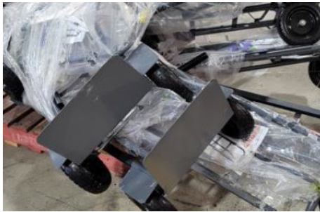
UNSUPPORTED & TOP HEAVY PALLETISED FREIGHT
