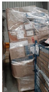
UNSUPPORTED & TOP HEAVY PALLETISED FREIGHT
